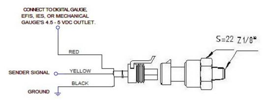
(Sender can be used to hook up to any gauge as long as it has a 4.5-5 VDC outlet.)
